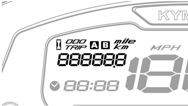
Press ADJ button to display ECU Working Time - Digital Clock Adjustment – ODO - TRIP A - TRIP B in cycles.
