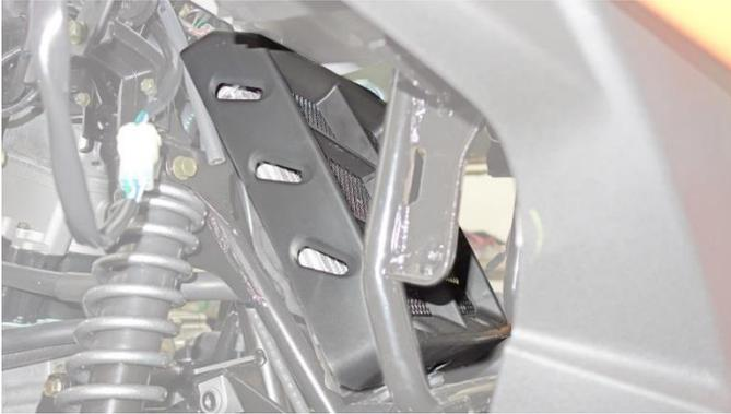
Periodically check the radiator area for cleanliness. Inspect radiating fins. They must be clean, free of mud, dirt, leaves and any other deposit that would prevent the radiator to cool properly. Remove as much as you can with your hands. If water is available in proximity, try rinsing the radiating fins. If available, use a garden hose to rinse the radiating fins.
