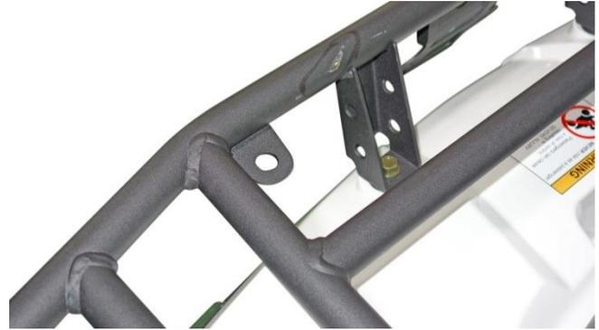
The rear rack of your ATV is equipped with a flag pole bracket. Flag poles are optional equipment available from your KYMCO dealer. Mounting a flag pole to your ATV, via the flag pole bracket, increases your visibility during operation.
