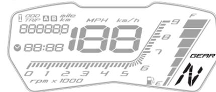
2. Turn the ignition switch to "ON" and check the neutral indicator lamp comes on.
