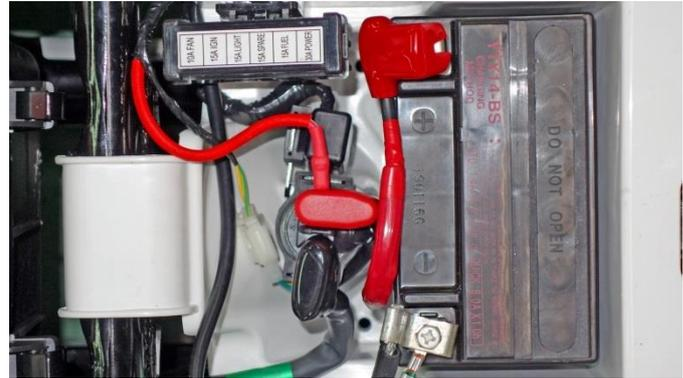
The battery is a sealed type, so it is not necessary to check the electrolyte level or add distilled water. If the battery is weak, see your KYMCO dealer for advice, for battery charging or replacement. If you replace the battery, select one that is sealed and is equivalent to the original battery in size and capacity.
