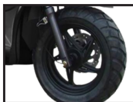
DUAL PISTON FRONT DISK BRAKES
