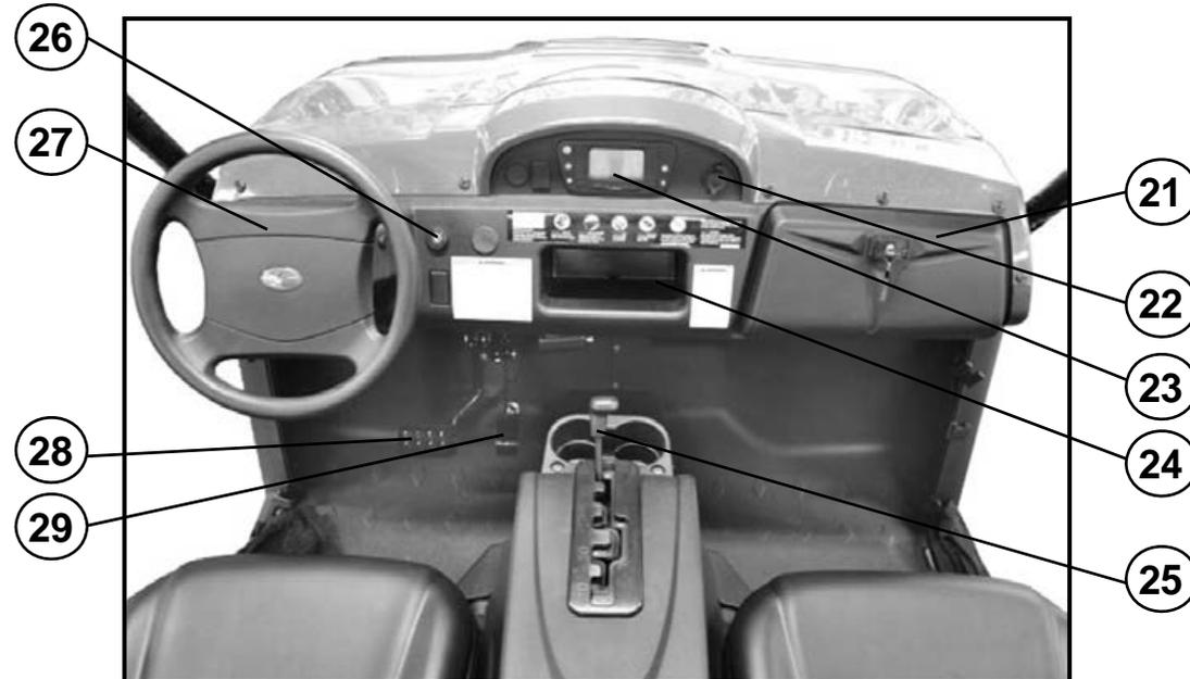
21.Right Glove Compartment 22. Auxiliary Outlet 23.Speedometer
