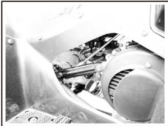
C. Remove the dipstick and wipe it off with a clean rag. Insert the dipstick in the filler hole without screwing it in.
