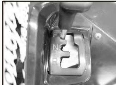
2. To shift into reverse gear, pull out and push downward on the shift lever until the transmission engages the reverse gear when the ignition switch is at the **ON** position, the reverse indicator light will illuminate.
