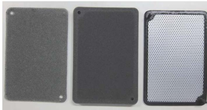
9. Gently wash the air cleaner elements in clean, non-flammable (high flash point) solvent such as kerosene —not gasoline. Allow the air cleaner to dry thoroughly before applying oil. A wet air cleaner will not fully absorb the oil.
