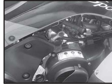
2. To shift into reverse gear pull out and push downward on the shift lever until the transmission engages the reverse Gear③ . When in the with the ignition switch in the **ON** position the reverse Indicator light will illuminate.④
