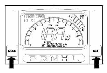
When you seeing clock position is flash word . You can start setting hour item. Press button B adjust correct hours then Press button A you can see minute position is flash. adjust correct minute. Waiting for 2second .finish times setting.
