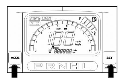
Press and hold button A and B until 5 seconds over . when at ODO function then you can see clock position is flash word .
