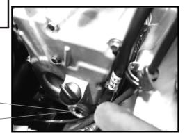
Engine oil replacement and oil filter cleaning
