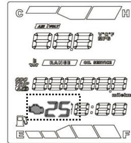
**NOTE:** If any error codes show up for a moment then goes off and not repeat, it could result from an electrical interference.
