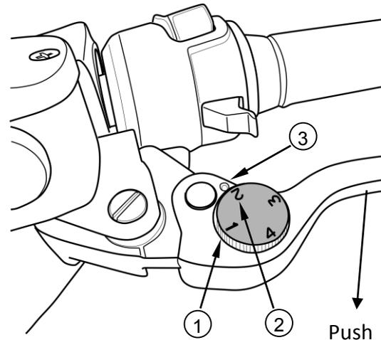
**NOTE:** The nearest distance from the grip to the released lever is set at number 1 and the farthest is set at number 4.
