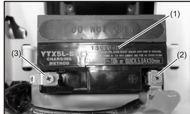
(1) Battery (2) Positive (+) terminal lead (3) Negative (-) terminal lead
