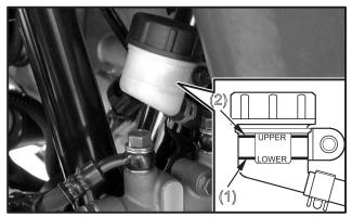
(1) Lower level mark (Foot brake pedal)(2) Upper level mark (Foot brake pedal)
