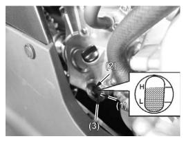
(1) Engine oil inspection window(2) Maximum level mark (H)(3) Minimum level mark (L)
