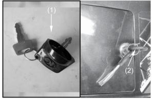
(1) Ignition switch keys (2) Right storage compartment lock and open keys
