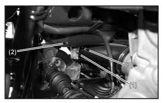
(1) Drain tube(2) Air cleaner housing(3) Clip
