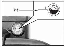
(1) Lower level mark (Hand brake lever)
