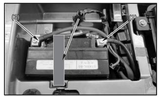
(1) Rubber band(2) Negative terminal lead(3) Positive terminal lead
