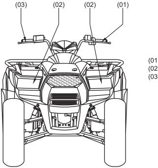
(01) Rear brake lever(02) Headlights/Position lights(03) Front brake lever
