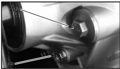
(2) Oil filler cap(3) Oil level check bolt/washer
