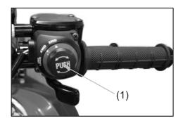
(1) 2WD/4WD select switch and differential lock switch
