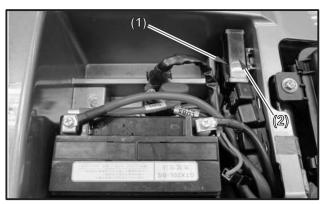
(1) Fuse box (2) Fuse box cap
