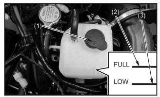
(1) Coolant reservoir cap(2) Maximum level mark(3) Minimum level mark
