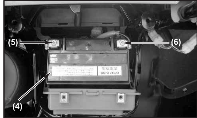
(4) Battery (5) (-) terminal lead (6) (+) terminal lead
